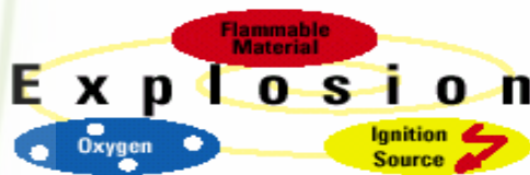
Figure 8.3 Explosion / Fire triangle
